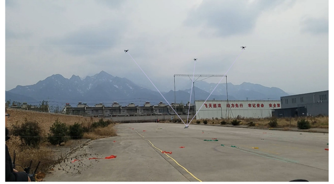
Fig. 1. Three tethered UAVs collaboratively transporting a payload.
